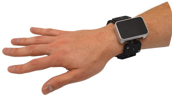
Fig. 1. Tasbi is a multisensory haptic wristband capable of delivering squeeze and vibrotactile feedback for a variety of uses in AR/VR.
